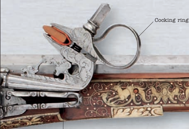
Spring holds cock firmly against striking wheel
