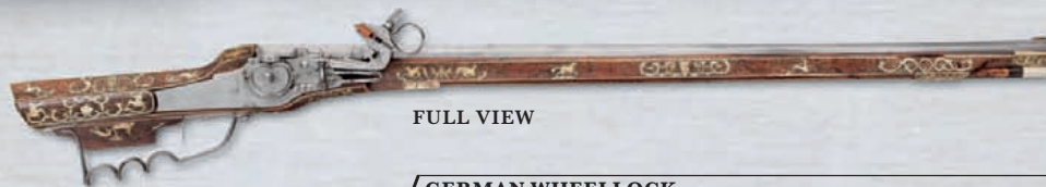
Spring holds cock firmly against striking wheel
