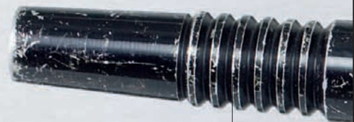
Rifle barrel has cooling fins
