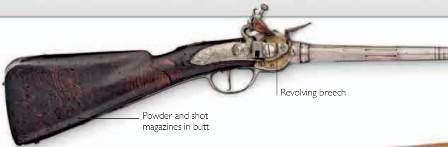
▲ ITALIAN REPEATING FLINTLOCK Date c.1690 Origin Italy Barrel 89cm (35in) Calibre 13.5mm (.53in)
