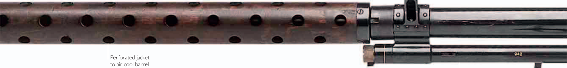
▲ SOLOTHURN S18-100 ANTI-TANK RIFLE Date 1930 Origin Switzerland Barrel 90cm (35½in) Calibre 20mm Armour penetration 35mm (1½in) at 100m (109 yards)
