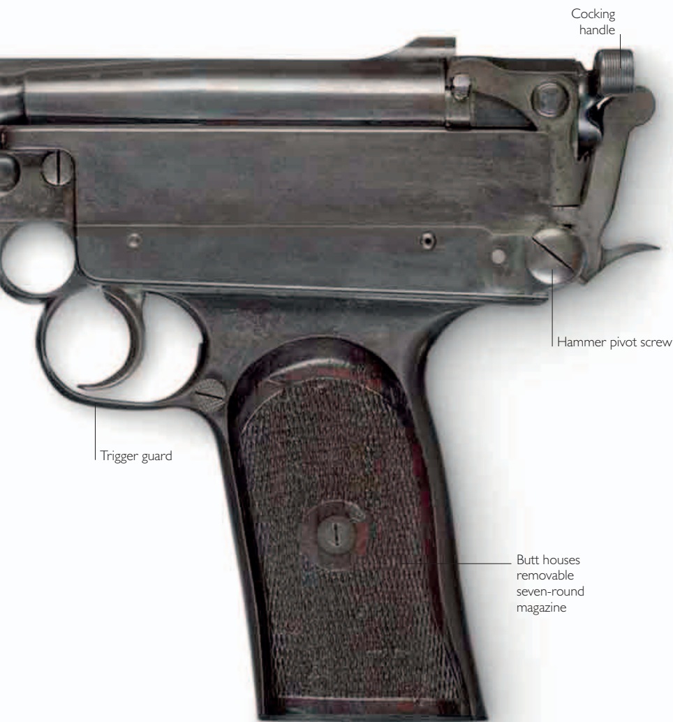
▲ BERGMANN NO. 3 Date 1896 Origin Germany Barrel 11.2cm (4½in) Calibre 6.5mm Bergmann
