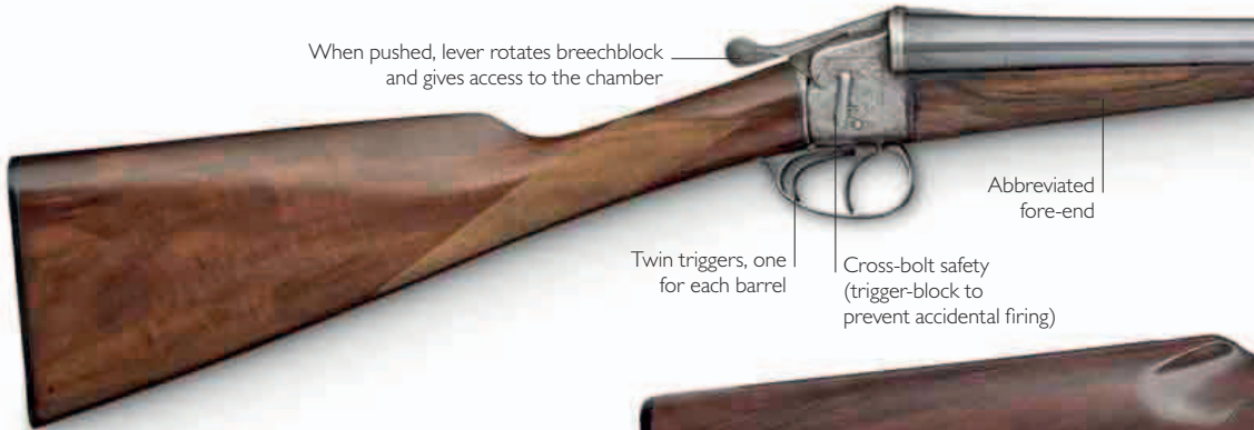
▲ DARNE ROTARY-BREECH SHOTGUN Date 1965 Origin France Barrel 65cm (25½in) Calibre 16-bore (16.76mm)
