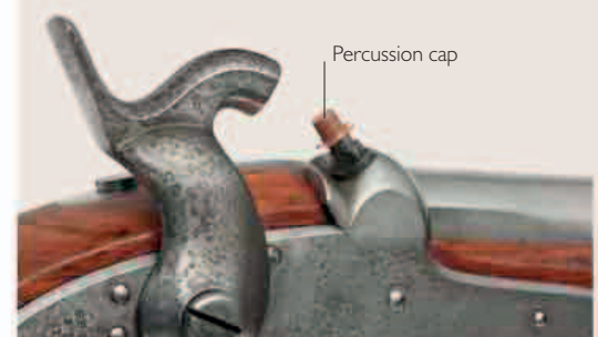
THE PERCUSSION CAP MECHANISM
